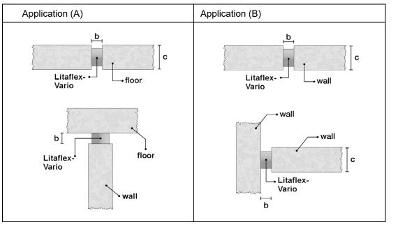
c thickness of the building element (rigid floor  $c_D$  or rigid wall  $c_W$ )
